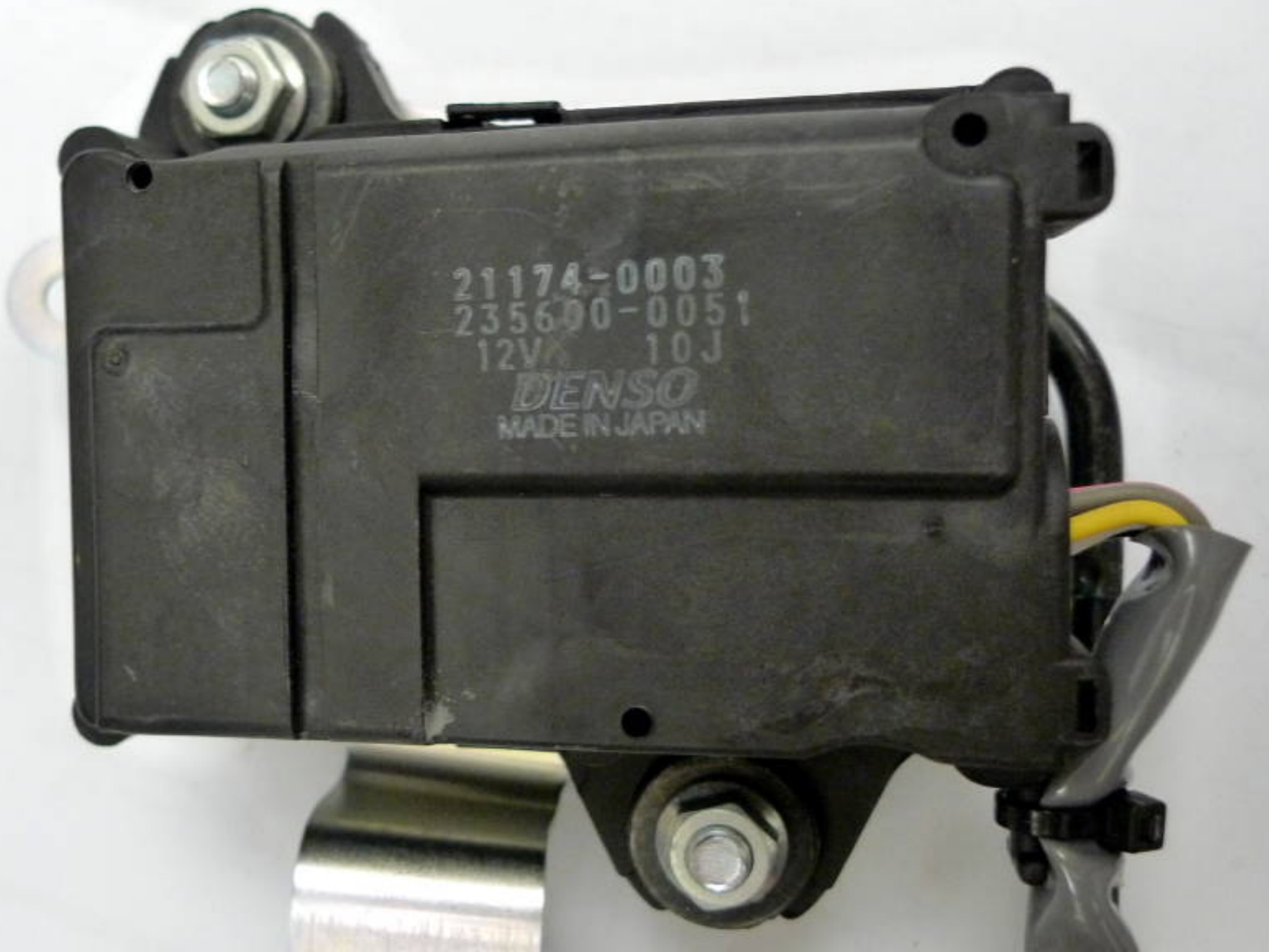
... similar to GSXR600/750 servo 320g (without bracket) - GSXR1000 servos complicated by a vacuum/pressure switch (not required)
