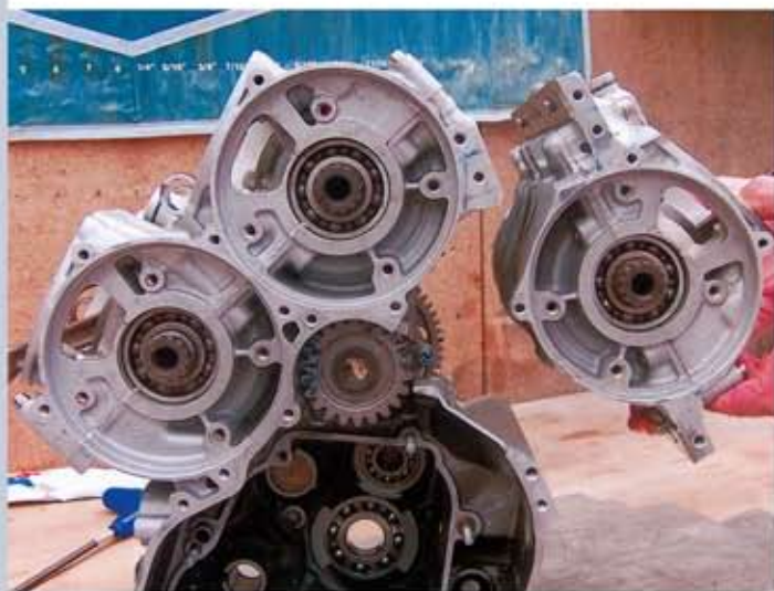
The extra cylinders bolt to the bottom of the engine via the pilot shaft
