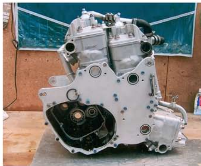
Additional cylinders mounted and side plate fitted for strength
