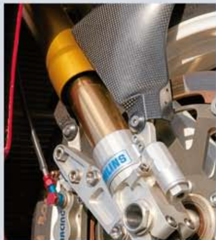
GP-spec Ohlins forks compliment the AP Racing six-piston callipers
