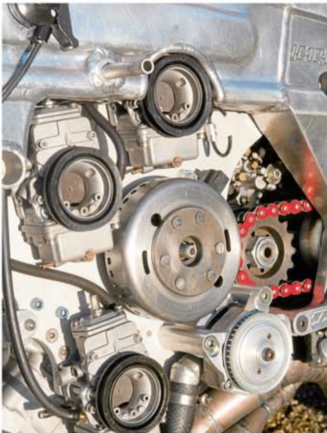
A Swiss-Auto water pump replaces the standard Suzuki pump
