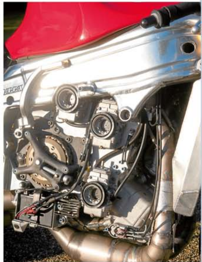
The dry clutch vies for attention with the carbs and pipes
