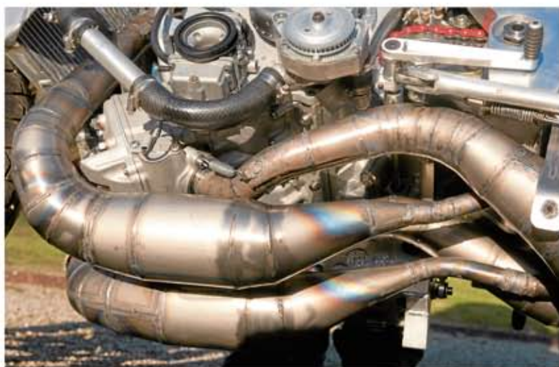
A snakes wedding of titanium pipes. Note GP-style exhaust flanges
