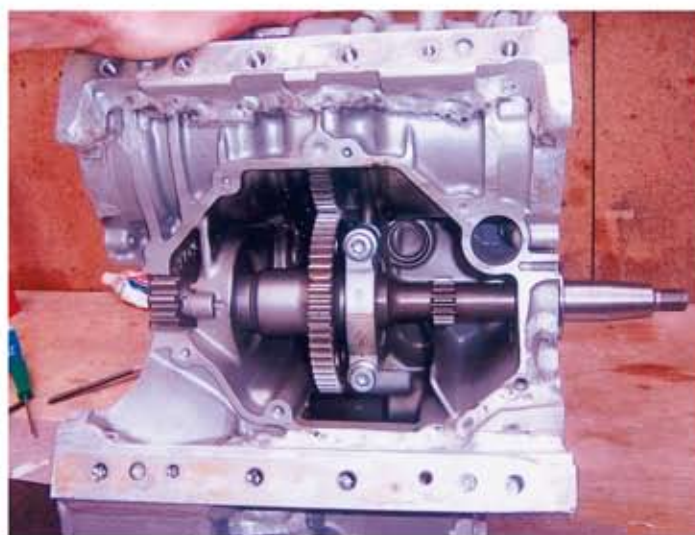
The pilot shaft gears all the cranks together and is machined from solid
